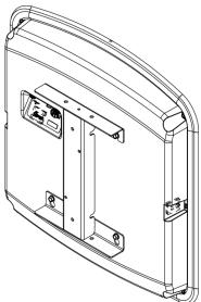
The display sign is equipped with an aluminum mounting support and stainless-steel flange bolts, allowing for quick and simple post installation.
